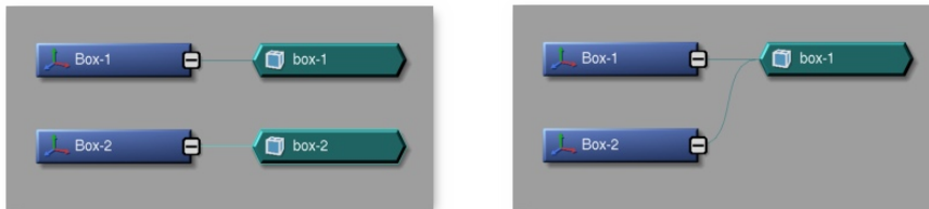
Figure 2.2. Schematics view of a duplicated (left) versus instanced (right) Object. The two situations will look identical on a 3D view, except when you edit the Mesh called “box-1” in the second case, both of its instances of it will change.
